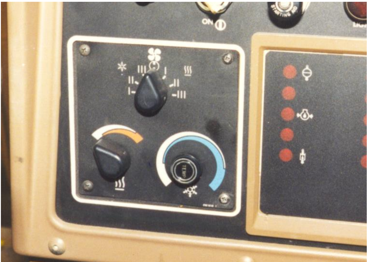
Thermostat in location on dash control panel.
